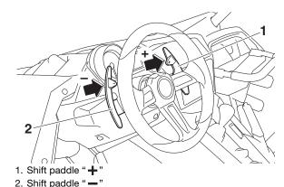
Use the shift paddles to shift through the forward gears. Pull and release the shift paddle "+" to shift up. Pull and release the shift paddle "-" to shift down.
