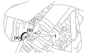
1. Headlight beam adjusting screw
