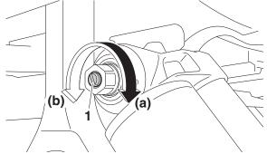
1. Low speed compression damping force adjusting screw
