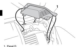
Turn the panel lock 1/4 turn counterclockwise, and then push the tab on the panel lock down so that it is pointing rearward.
