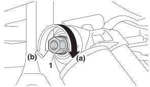
1. High speed compression damping force adjusting bolt
