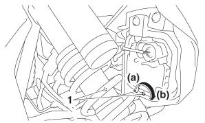
1. Headlight beam adjusting screw
