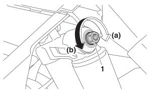
1. High speed compression damping force adjusting bolt
