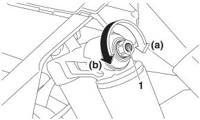
1. Low speed compression damping force adjusting screw
