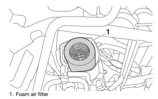
3. Remove the foam air filter element from the air filter frame.
