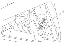
1. Engine oil tank filler cap
