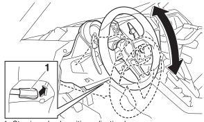
1. Steering wheel position adjusting lever
