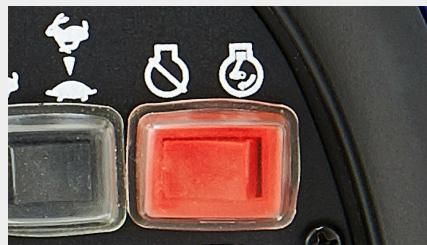
**Smart Throttle™ load-sensing throttle control**
