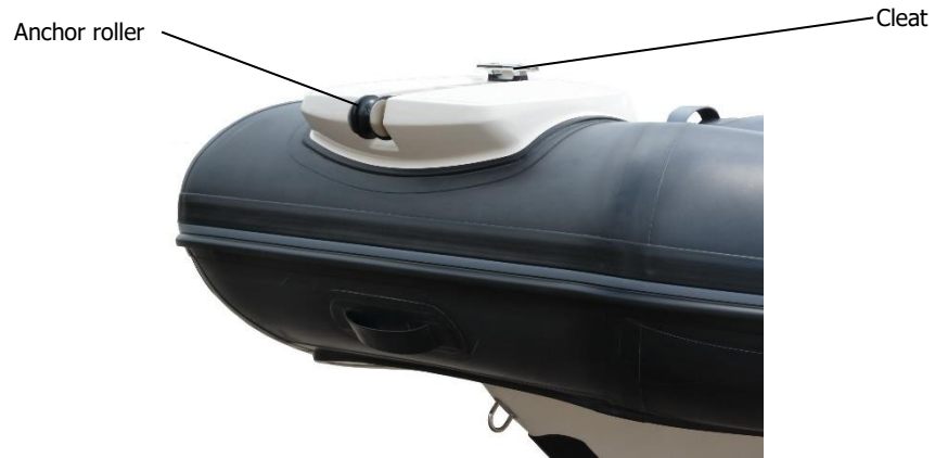
Fig. 32. Bow step plate.
