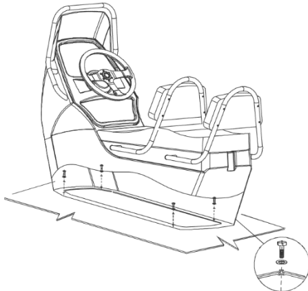
Fig. 7. Installation of steering console CS-03.
