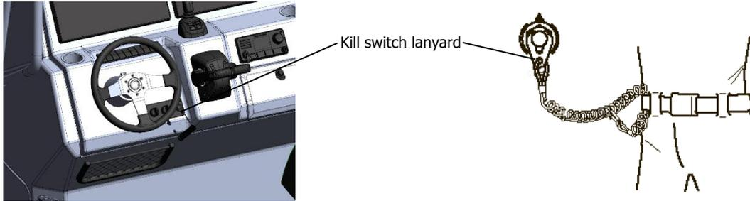
Fig. 28. Engine kill switch lanyard.
