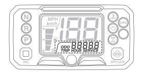
Push the select button "SEL" to switch the display between the odometer "ODO", the tripmeter "TRIP", the service tripmeter "SERVICE", and the hour meter "HOUR" in the following order:
