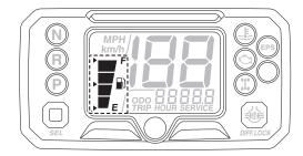
The fuel gauge indicates the amount of fuel in the fuel tank. The display segments of the fuel gauge disappear from "F" (full) towards "E" (empty) as the fuel level decreases. When the last segment starts flashing, refuel as soon as possible.
