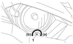
1. Headlight beam adjusting screw
