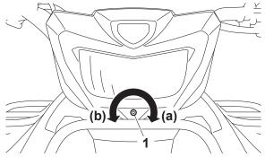
1. Handlebar-mounted light beam adjusting screw
