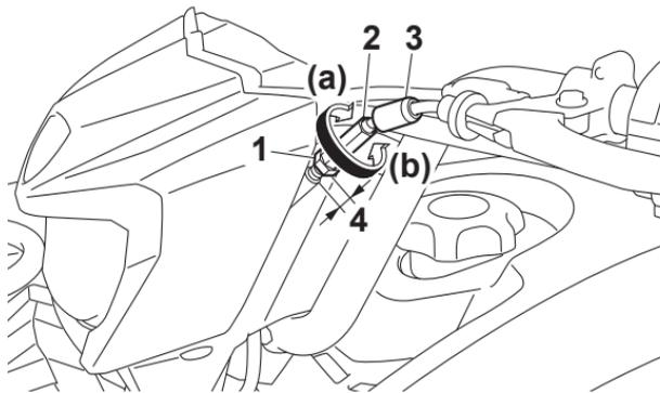
1. Brake cable adjuster locknut
