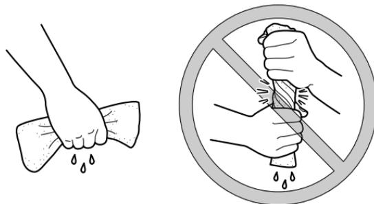
8. Check the air filter elements (sponge material) for damage, replace if necessary.
