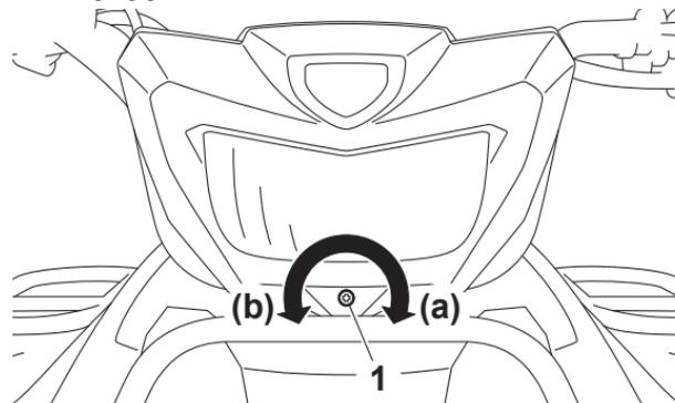
1. Handlebar-mounted light beam adjusting screw
