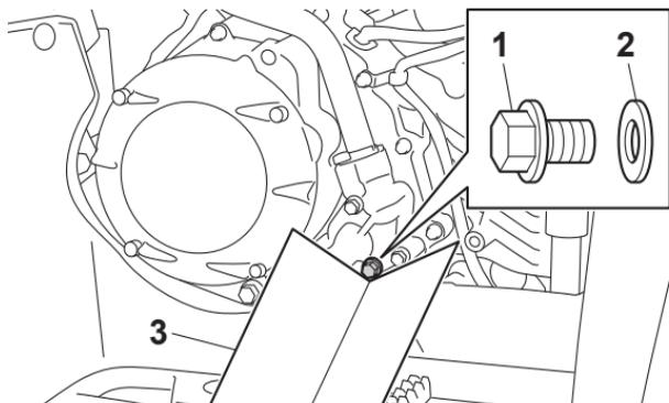
1. Coolant drain bolt
