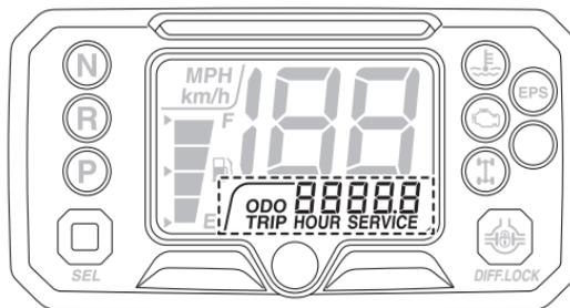
Push the select button "SEL" to switch the display between the odometer "ODO", the tripmeter "TRIP", the service tripmeter "SERVICE", and the hour meter "HOUR" in the following order: ODO → TRIP → SERVICE → HOUR → ODO
