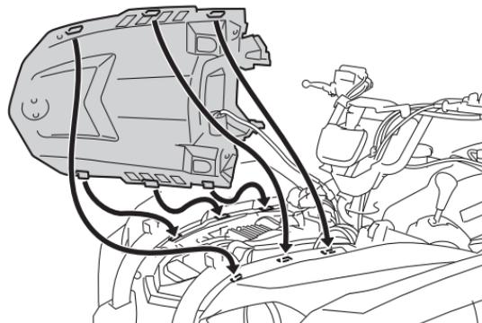
2. Install the quick fasteners.
