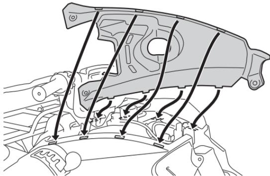
3. Install the bolts and quick fasteners.
