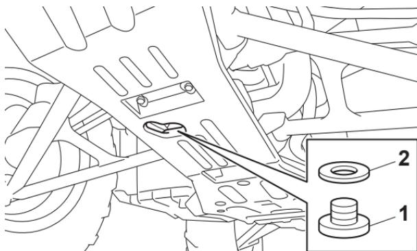
1. Differential gear oil drain bolt
