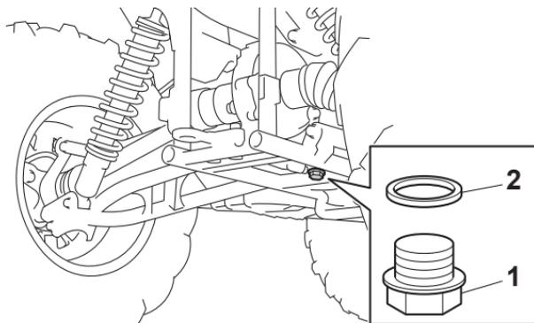
1. Final gear oil drain bolt
