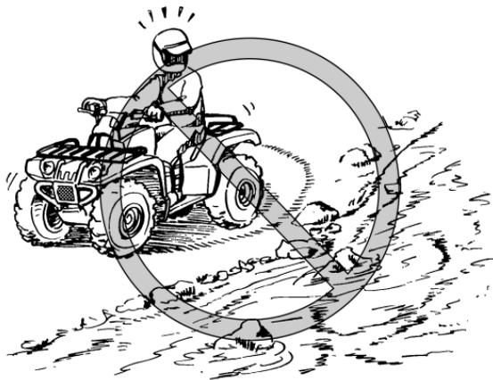
Test your brakes after leaving the water. If necessary, apply them several times to let friction dry out the linings. Do not continue to ride your ATV without verifying that you have regained proper
