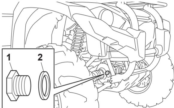
1. Differential gear oil filler bolt
