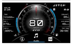
Smart features are accessed via the pop-up menu system at the bottom of the main display (see page 5-14). The menu system and all related features are controlled using the joystick/home button "50" (see page 5-2).
