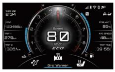
Operate the joystick up-down to cycle between grip warmer OFF and 3 presets which can be customized in " $\circledast$  Machine Settings"  $\rightarrow$  "Grip Warmer". (See page 5-25.)
