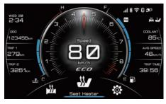
Operate the joystick up-down to cycle between seat heater OFF and 3 presets which can be customized in " $\circledast$  Machine Settings"  $\rightarrow$  "Seat Heater". (See page 5-26.)
