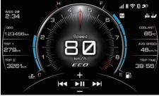
This opens a simplified version of the audio player. A full audio player is available by navigating to "M Applications"  $\rightarrow$  "Audio". (See page 5-20.) Operate the joystick up-down to adjust the volume. Operate the joystick left-right to skip to previous/next track. Short press enter " $\checkmark$ " to play/pause.
