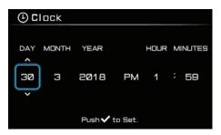
To manually adjust the clock, highlight items by operating the joystick leftright. Operate the joystick up-down to adjust the value of the highlighted item. Short press enter " $\checkmark$ " to set the clock and return to the previous menu.
