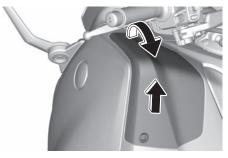
To install the panel Place the panel in the original position, and then install the screw.
