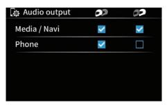
When a Bluetooth headset is connected, the headset icon "O" / "O" will appear on the top of the display. This setting module changes the media/navigation and phone call audio between the "Rider headset" "O" and "Passenger headset" "O".
