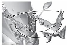
3. Install the quick fasteners.
