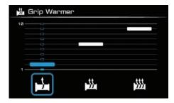
The three grip warmer presets can be customized here. Select a preset by operating the joystick left-right and adjust its heat level from 1-10 by operating the joystick up-down. Confirm the settings by short pressing enter " $\checkmark$ " and return to the previous menu.
