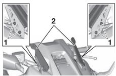
1. Bolt 2. Bracket Install the bracket to the high position by installing the bolts, and then tighten the bolts to the specified torque. WARNING! A loose windscreen could cause an accident. Be sure to tighten the screws to the specified torque.
