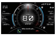
When a phone call is received to a connected smartphone, the ringtone will play through the connected headset and a telephone function will appear at the bottom of the display. Short press enter " $\checkmark$ " on the green phone icon to
